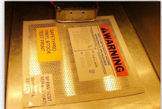
ISS materials are tested for label life under intense UV exposure
