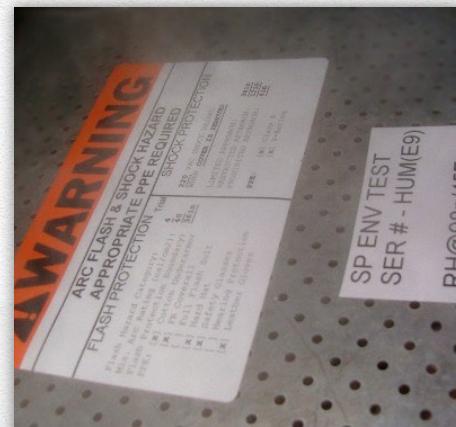
Humidity testing helps determine label adhesion in humid environments
